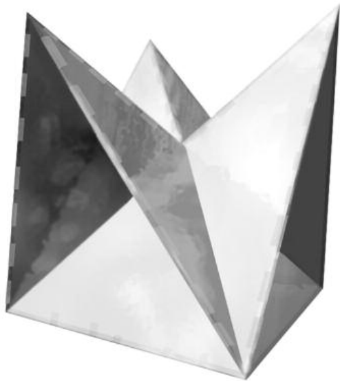
An illustration of a typical Project Mogul radar reflector, constructed from aluminized paper over a balsa wood frame.
